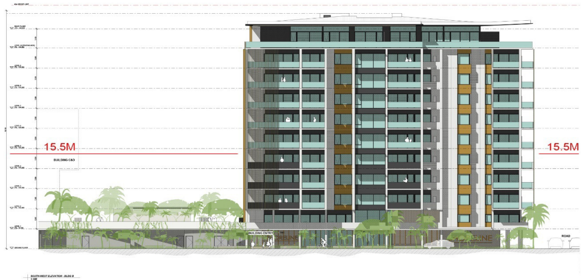
Figure 6: Detailed Elevation showing height of Building B relative to 15.5m standard
