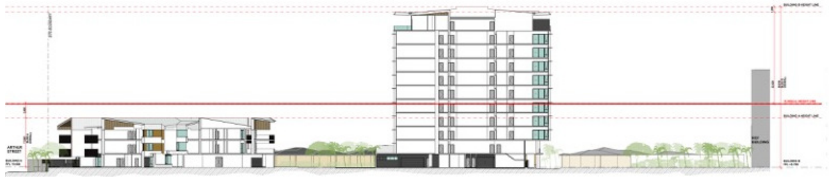
Figure 5: Elevation showing height of Building a and B relative to 15.5m standard
